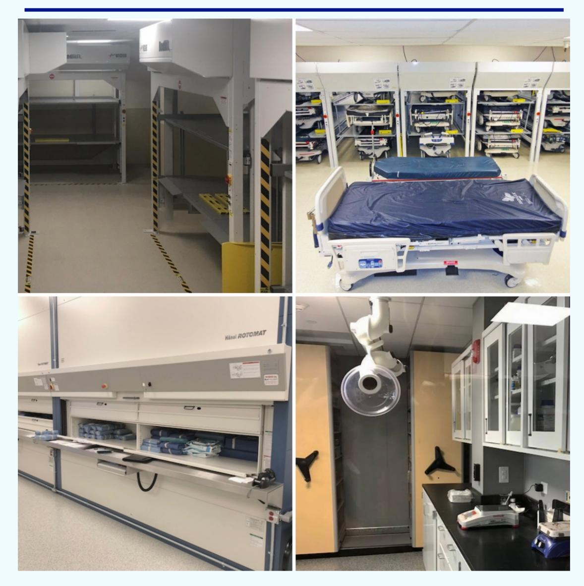
Non-traditional solutions can include automated vertical storage and mobile aisle storage. Both create solutions that reduce the footprint of shelving whether by building upward to utilize vertical space (including multi-floor solutions) and mobile aisle storage, which eliminates all but a single 'moveable' aisle.
