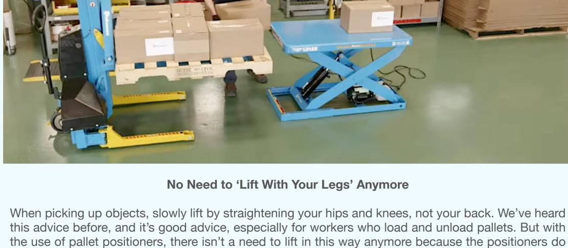
Pallet positioners allow workers to ergonomically load and unload pallets by moving work to the employee—not the other way around. The positioners automatically adjust their height as items are
